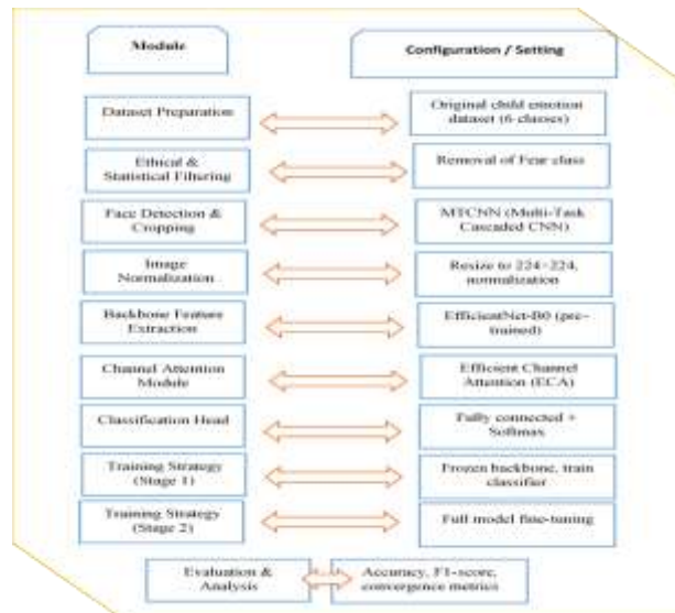
Figure 2. Proposed Facial Emotion Recognition Architecture and Experimental Flow
